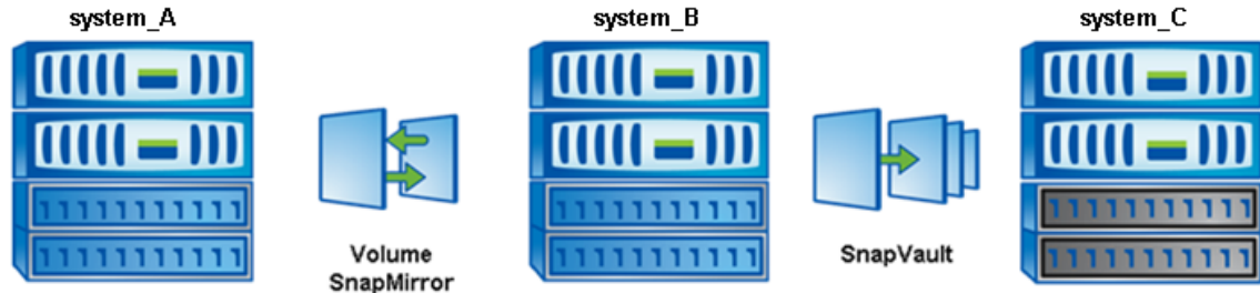
Figure 4) Protecting a volume SnapMirror destination with SnapVault.
