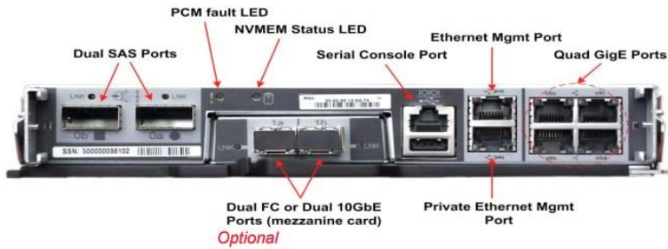
Figure 3) PCM showing indicator LEDs, standard ports, and optional ports on mezzanine card.
